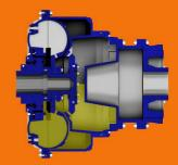
**IDELE POSITION:** The operating fluid remains static inside the coupling.
