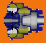
**START UP:** The driving machine provides the energy to accelerate the operating fluid in order to generate a roundabout current. Due to the transmission of the kinetic energy by the fluid, the internal wheel (turbine wheel) is put in motion.
