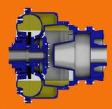
**NORMAL OPERATON:** During normal operation only the torque required by the driven machine is transmitted by the coupling, which is designed to absorb possible overloads without passing these on to the drive.
